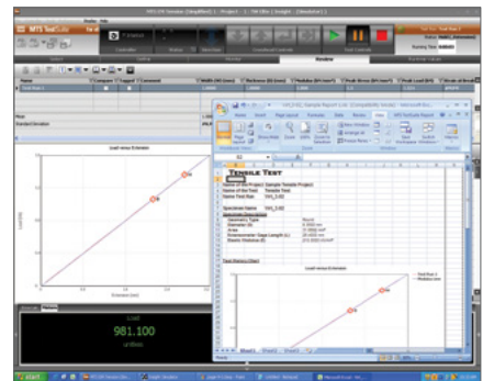
Integrated runtime reporting capabilities allow you to efficiently export test results to Excel and ASCII formats.
