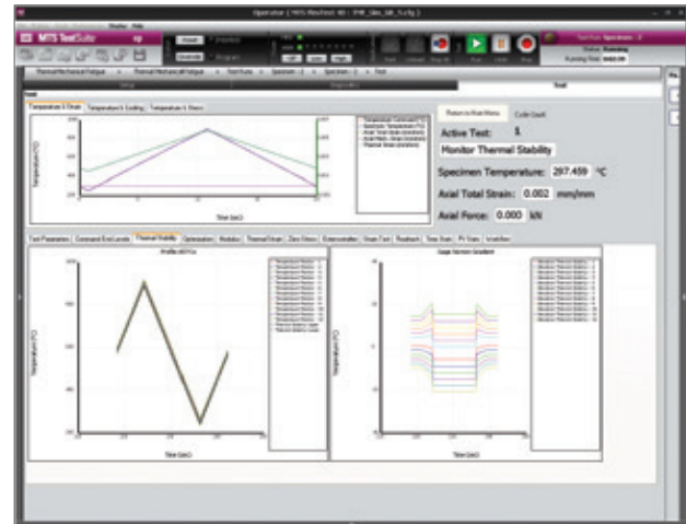
The Runtime View of thermal stability at batch level offers simple validation that the temperature gradient has been achieved
