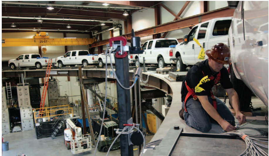
Innovative civil engineers at the University of Nevada, Reno NEES Equipment Site investigate the seismic effects of multi-span curved bridges using a 2/5 scale model of a three-span bridge.
