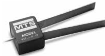
Standard equipment includes the gage and storage case, two reusable hardened knife edges for attachment to the specimen, and an instruction manual.
