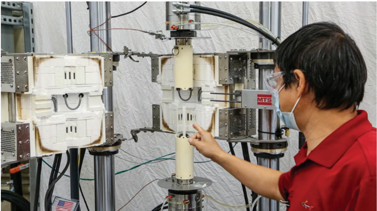
High-temperature testing solution with Model 680.15 grips and a 3-zone furnace
