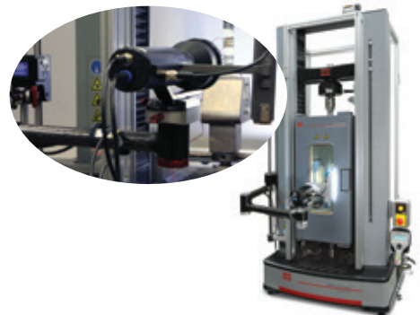
Non-contacting Video Extensometer
