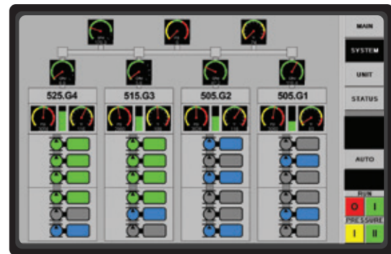
Multi-Pump Control Manager (MPCM)
